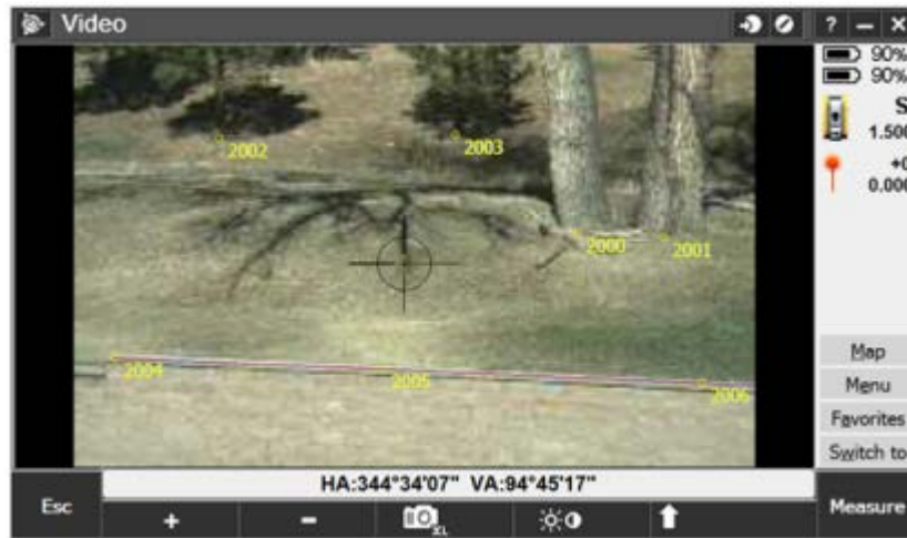
Figure 13. Trimble Access with overlay cross-hairs and survey data on the video feed
