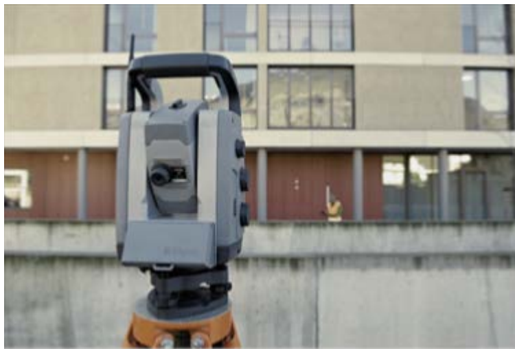
Figure 12. Trimble Access being used to remotely measure points in the field
