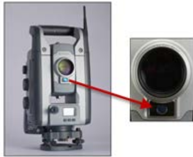
Figure 1. Total station with Trimble VISION camera
